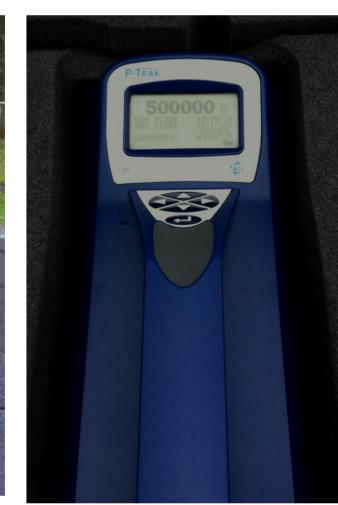
Even new low-emission stove under optimal operation pollutes above the upper detection limit (500,000 part/cm³)
