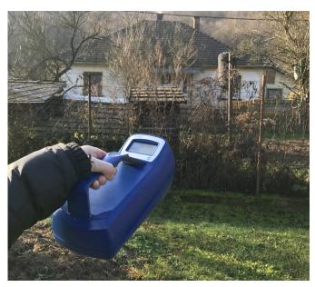
The project team conducted many outdoor measurements with an ultrafine particle counter.
