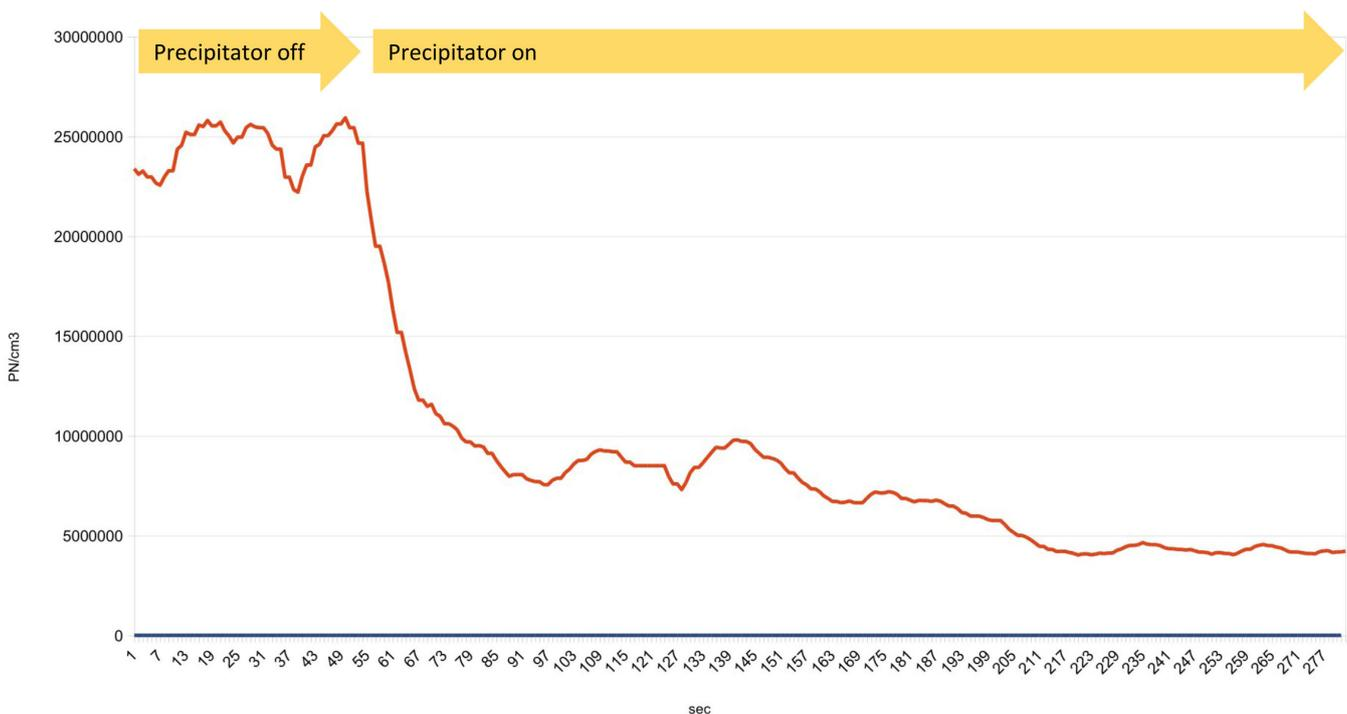
Figure 3: Our measurements showed that number of particles emitted can be reduced substantially by retrofitting a pellet boiler with a precipitator.
